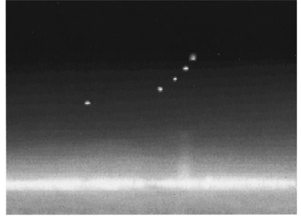
FIG. 4. Superimposition of five CCD camera frames showing the levitation height increase of the same dust particle above a conducting plate (at the bottom of the figure) when the plate negative voltage is increased from -26.5 V to -32 , -38 , -44 , and -50 V.
